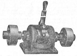
The Gears are always in mesh, run in oil, and any degree of friction can be obtained by a simple adjusting feature.
