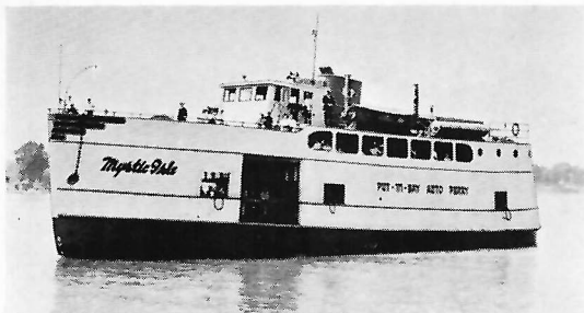
Serving the traffic from Catawba Point to Put-in-Bay, the 110-foot MYSTIC ISLE, built by Berger Boat Company at Manitowac, driven by two 6-cylinder Gray Marine Diesels.
